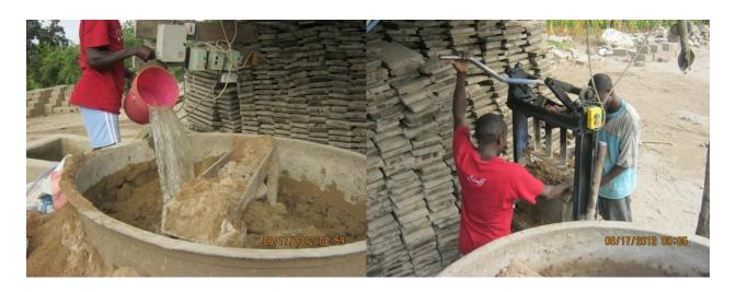
Figure 5: Production of sand cement blocks
